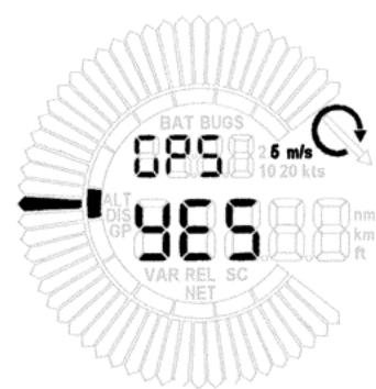
Fig. 16 GPS input active GPS data present
