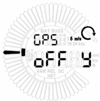
Fig. 13 GPS input not active GPS data present
