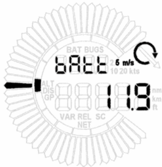
Fig. 29 Battery voltage display
