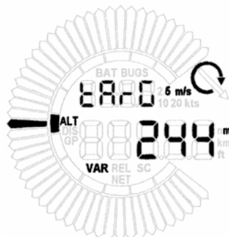
Fig 10 Landing place elevation input (target)
