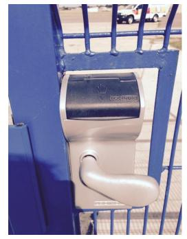
Lift open the black cover to reveal the buttons underneath and enter the code.
